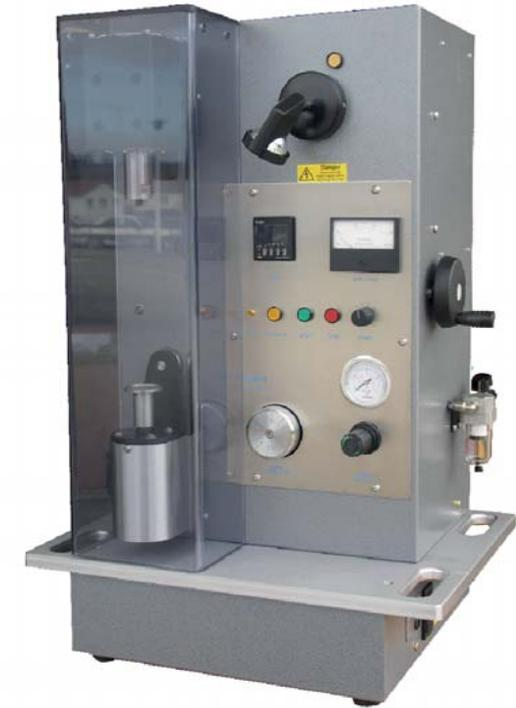
The machine can rapidly de-ring, reshape and if required, enlarge the bore of worn dies. But the primary purpose of this machine is final polishing.
