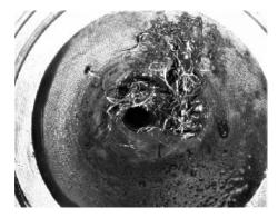
Friction against a sharp angle at the end of the bearing also causes small vibrations to the wire, which propagate inside the machine.
