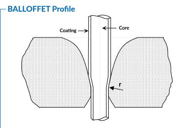
The internal profile must be geometric enough, in order to draw the wire core and the coating in an uniform soft way. This internal profile avoids the «sock effect», meaning the coating layer stretching.
