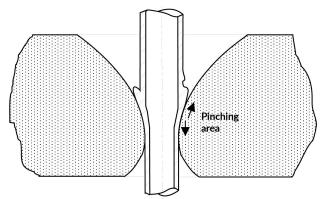
When the wire reduction is made on a too rounded profile, only the wire core will be drawn.
