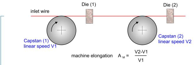
Elongation between the dies in adequation with the machine elongation: The wire runs perfectly
